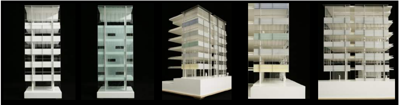
Façade studies exploring module proportions, frit banding and colour
